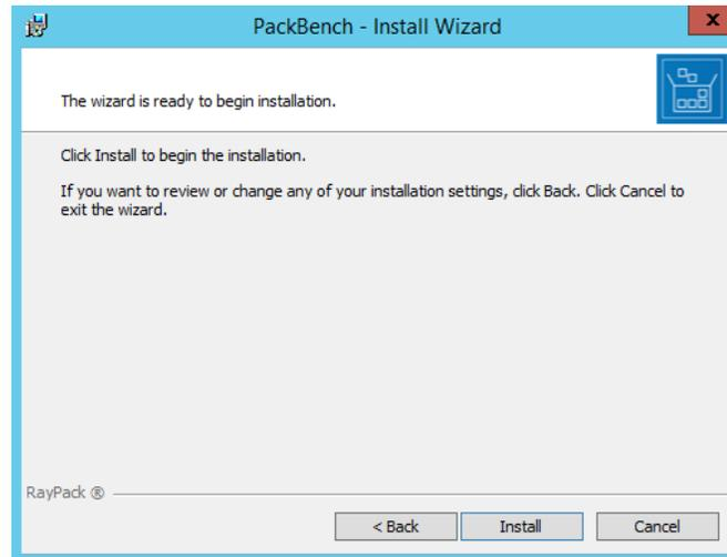
All required settings and properties are defined and PackBench is ready to be installed. Click **Install** to start the process.
